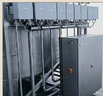
Metering technology for the filler lines
