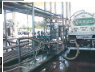
Reception station for raw milk from tankers
