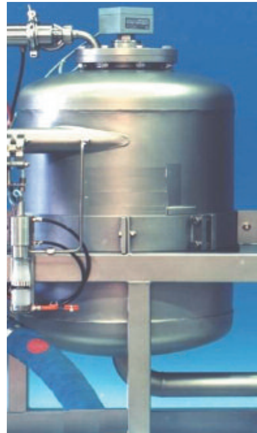
Air separator with continuous level measurement
