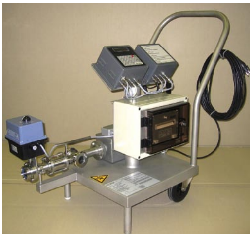
Figure 1: Mobile volumetric metering unit for automatic filling with print-out of an official voucher
