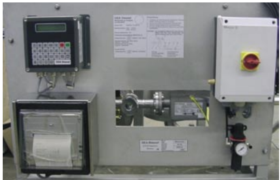
Figure 5: Measuring unit for tanker vehicles with main counter and printer
