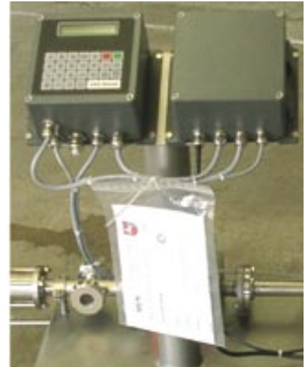
Figure 4: IZMTE metering system with integrated main counter (including official pre-test certificate for calibration)
