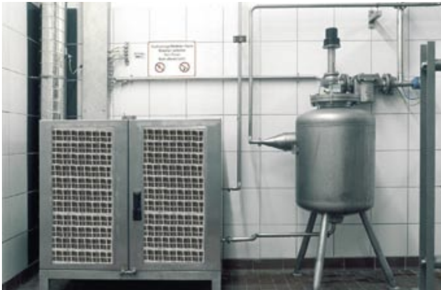
Figure 8: Completely sealed measuring section for alcohol
