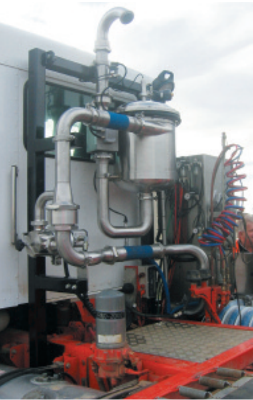
“FastSpeed” metering unit mounted on the tractor of an articulated vehicle
